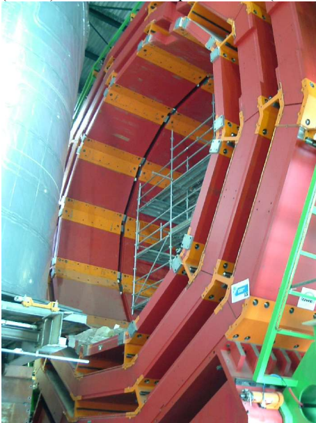
Fig(1.4.5.a) – Iron return yoke with spaces for muon chambers
