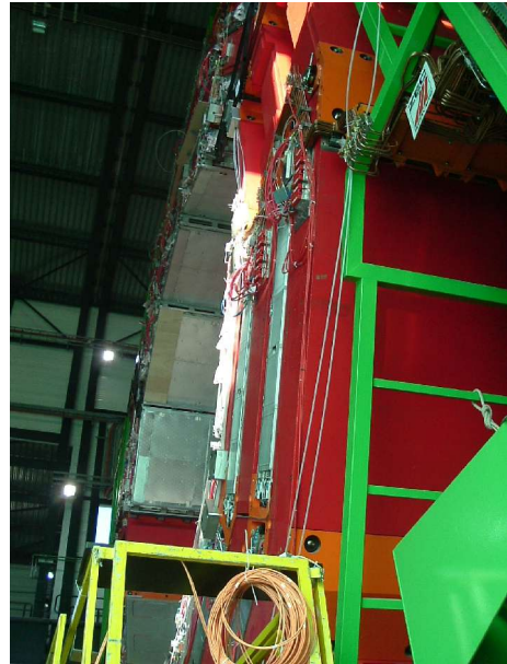
Fig(1.4.5.b) - Muon chambers installed between rings of iron return yoke
