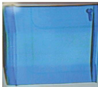
Figure 3 X-ray image of Box 3. This is one of the most conclusive images – it shows a small metal screw in the top right corner.
