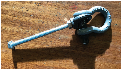
Figure 3. A bow shackle attached to the eye nut.
