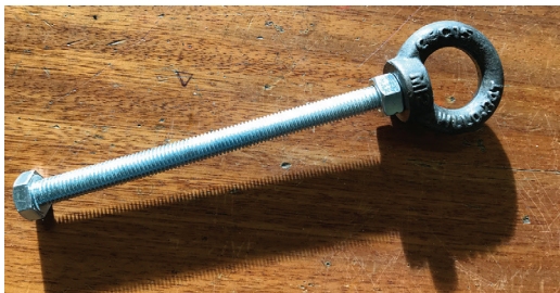
Figure 2. An 18cm M12 nut and bolt and an M12 eye nut. Shown without the ball for clarity.
