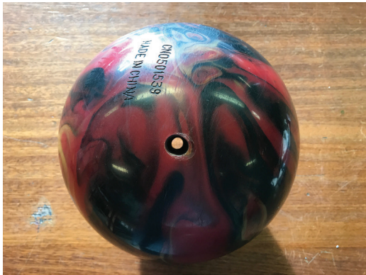
Figure 1. A 14mm hole drilled through a bowling ball.
