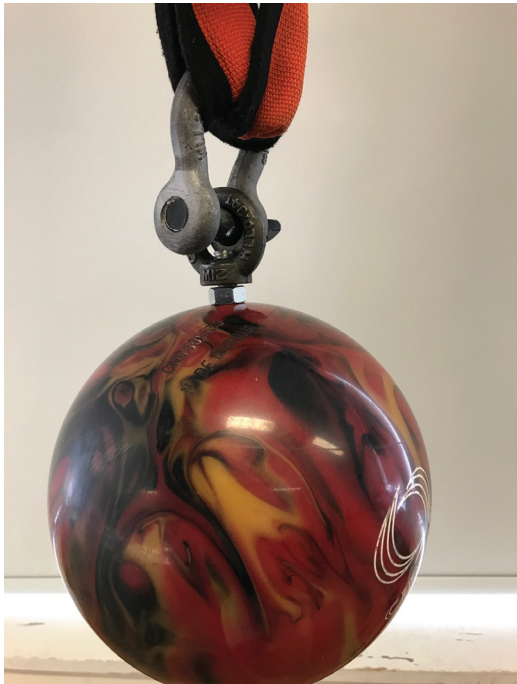
Figure 5. The bowling ball pendulum completed.
