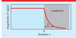
**Figure 1.** The exponential decrease of the magnitude of an electric field inside a conductor.
